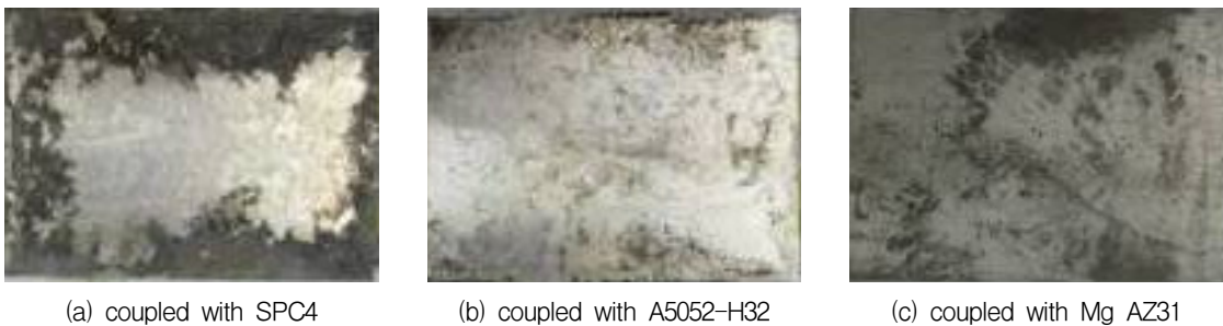
Fig. 2-4. Corroded surfaces of AZ31 Mg after immersion test for 72 hour in distilled water
