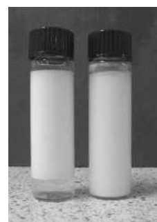
Fig. 4. An O/W, 20/80 emulsion (left hand tube) and A/O/W, 20/16/64; after 3 weeks storage at \sim 8^{\circ}\text{C} (taken from ref. 24).
