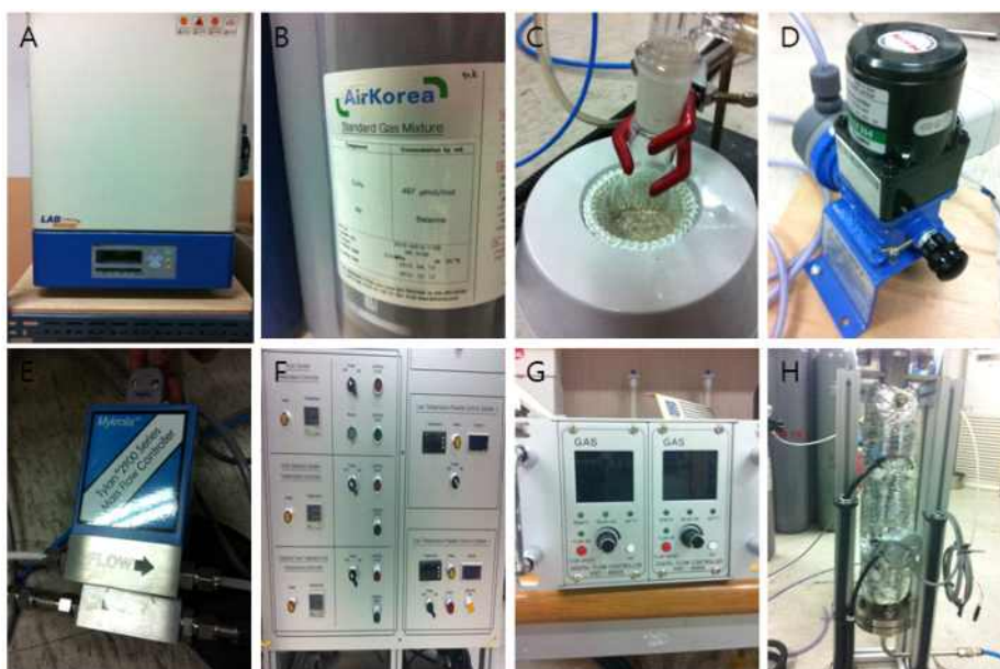
Fig. 4. Experimental equipments : Furnace (A) ; Toluene Gas (B) ; Toluene Bubbling Process (C) ; Chemical Feed Pump (D) ; Mass Flow Controller (E) ; PID Temp Controller (F) ; MFC Controller (G), Reactor (H).
