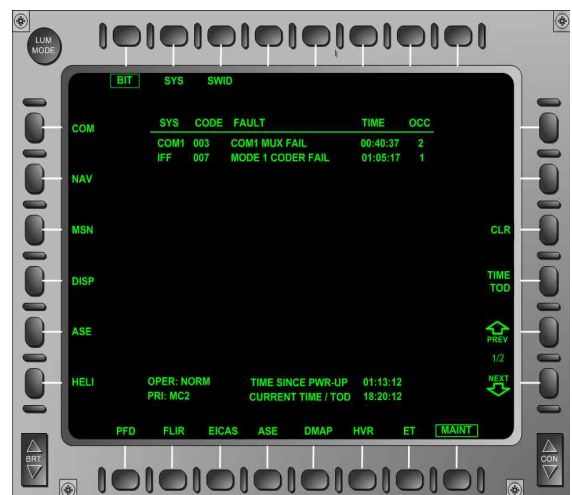
Fig. 2. Maintenance Fault List Page
