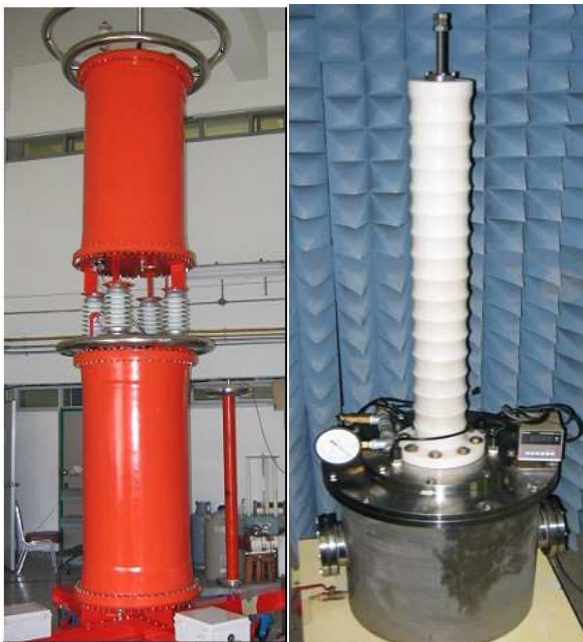
(a) AC high voltage source (b) The model GIS chamber
