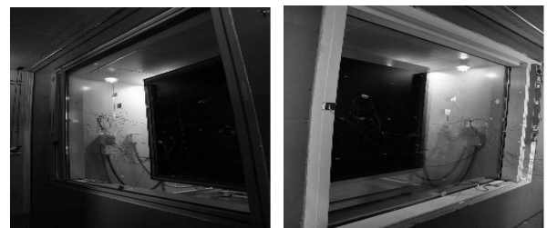
Fig. 2 Measuring U-factor of window.
