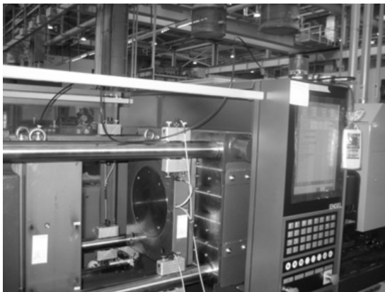
Fig. 5 Elongation test equipment set-up of tie-bar
