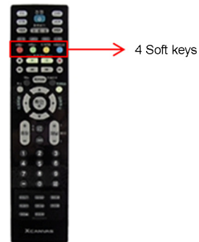
(b) 4 soft keys of a remote controller
