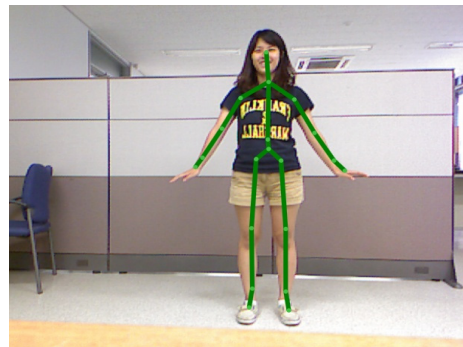
Figure 2. An example of human posture recognition by the KINECT sensor
