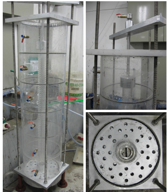
Fig. 3. Lab-scaled self-weight consolidation test equipment embedding vertical drain
