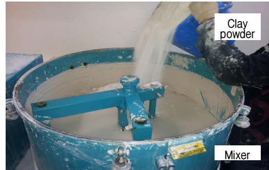
(b) Clay specimens using clay mixer
