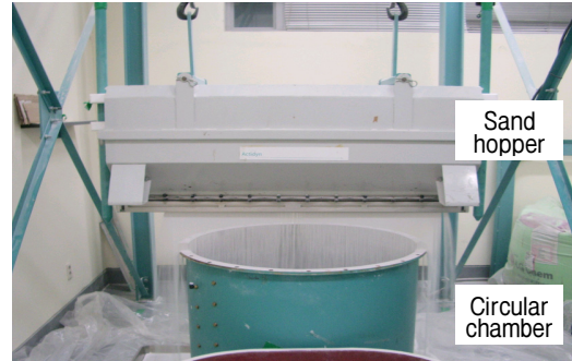
(a) Sand specimens with raining method with a sand diffuser
