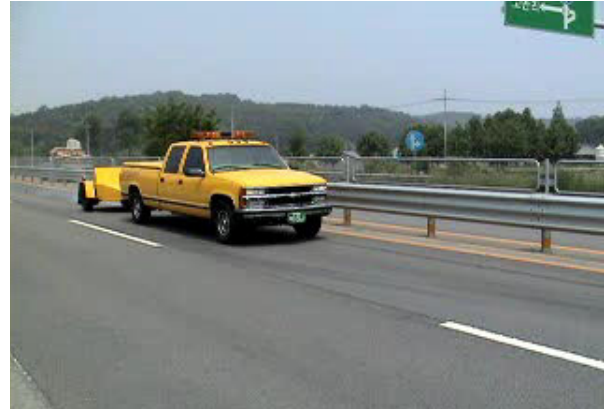
Fig. 3 Skid Resistance Measurement Scene
