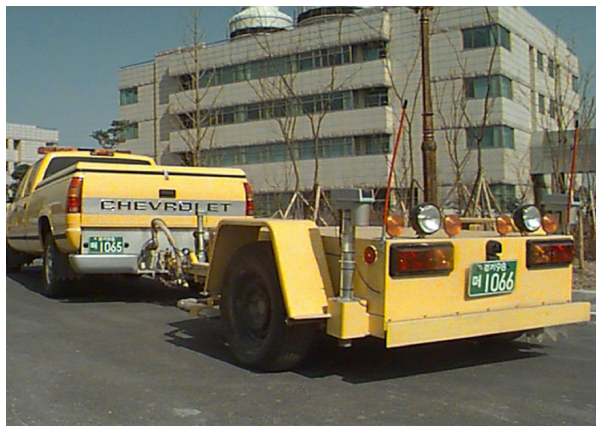
Fig. 2 Skid Resistance Measurement Equipment (Vehicle)
