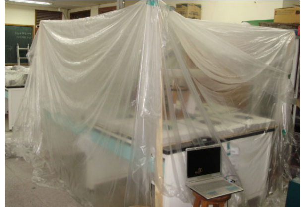
Fig. 9 Test Setup for Plastic Shrinkage Measurement
