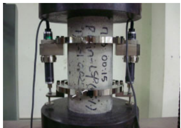
Fig. 10 Test of Elastic Modulus of Concrete Specimen
