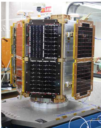
Fig. 4. Vibration test setup in x, y, z dir.
