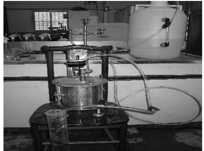
Fig. 2 Permeability test equipment
