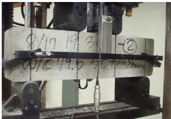
Fig. 1 Fracture Toughness Test Setup (ASTM C 1028)
