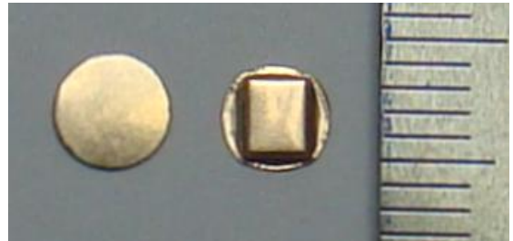
Fig. 4 Photograph of samples; (a) Blank, (b) Drawn cup
