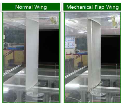
Fig. 8. Experiment setup for wind tunnel test of Normal wing and Mechanical Flap Wing( 0^\circ )
