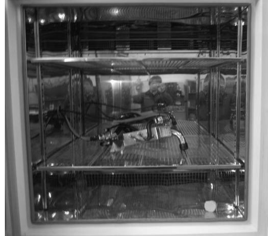
Fig. 11 Humidity durability test
