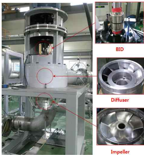
Fig. 7 Assembly of test pump
