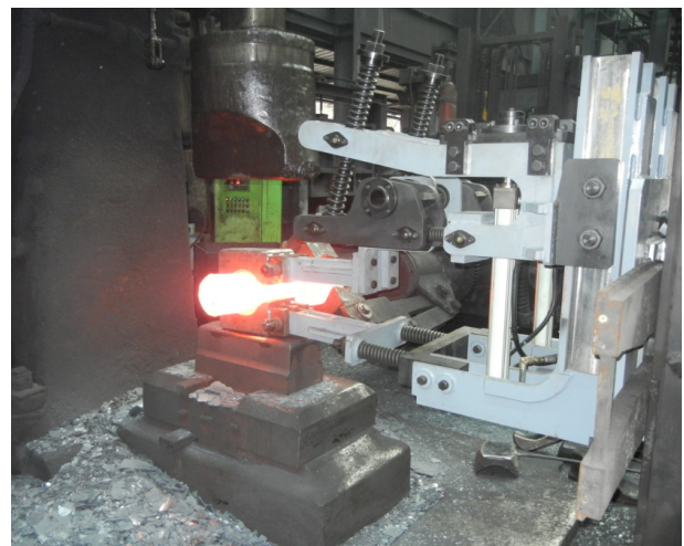
Fig. 7 Test production of 100 kg connecting rod
