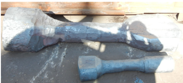
Fig. 9 Compare the size of 100 kg and 1,500 kg connecting rod
