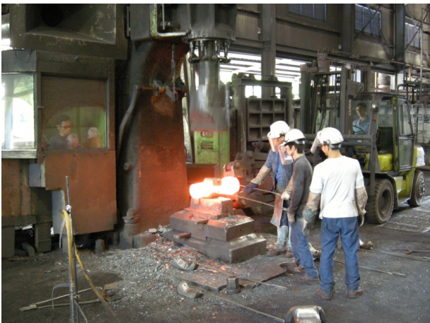
Fig. 1 Open die forging process
