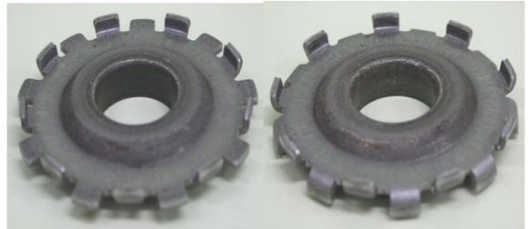
Fig.14 Analysis results for bending punch angle
