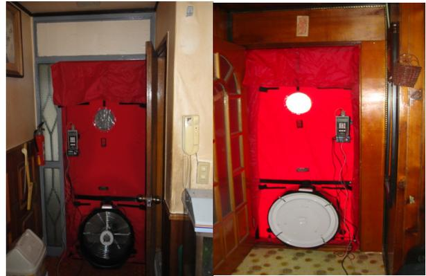
Fig. 1 A field test using by Blower Door.
