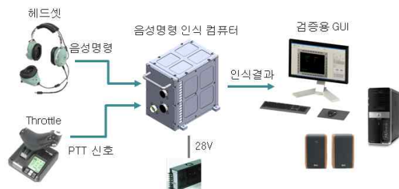
Fig. 1. Architecture of Voice Command System
