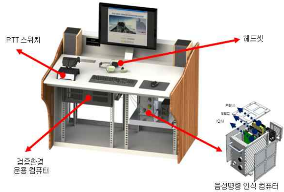
Fig. 5. Configuration of Verification Environment
