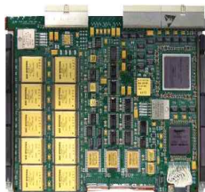
- BAE RAD750 SBC - (성능 : 260 MIPS @132MHz IF : SpaceWire, 1553B, UART, PacketWire, OBDH, CAN, PCI)
