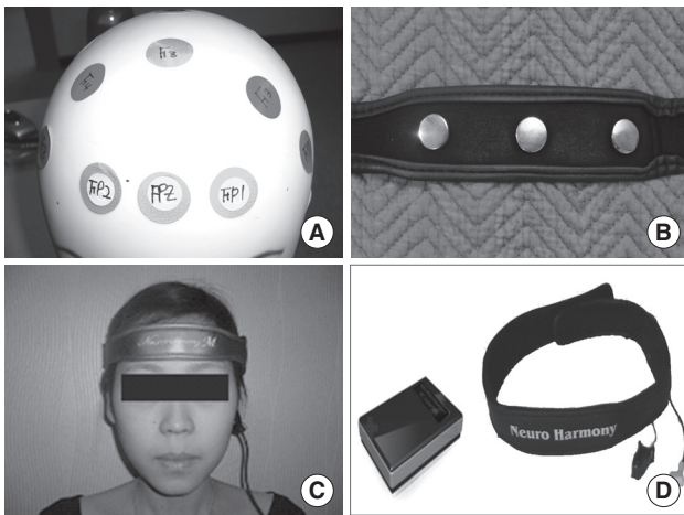
Figure 1. Brain computer interface. (A) Position of Fp1, Fpz & Fp2. (B) Dry terminal inside the head band. (C) Standard electrode of earlobe. (D) Brain wave measurement device
