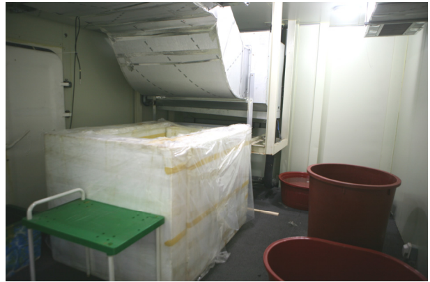
Fig. 2 A miniature tank and some dummy buckets for control of air temperature in cold room
