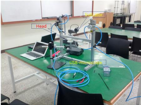
Fig. 13 Experimental apparatus for a simple air-chucking test
