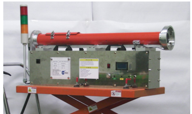
Fig. 2 Photograph of fabricated safety fence performance tester
