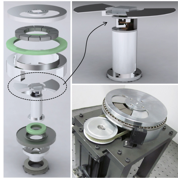
Fig. 7 Magnet wheel shielded partially with a separate actuator varying the open area of the shield plate
