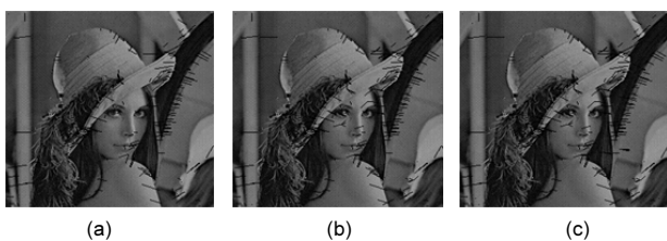
Fig. 9. Features detected by scale invariant feature transform algorithm with a changing number of scales. (a) 2 octaves, (b) 3 octaves, and (c) 4 octaves.
