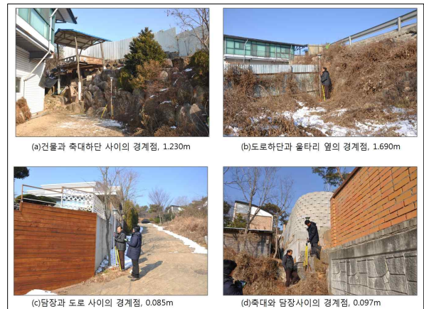
Figure 5. Case of exceeding the allowable error tolerance( \pm 0.07m ) in residential area
