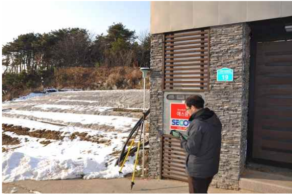
Figure 6. Large observation error due to buildings (0.085m)
