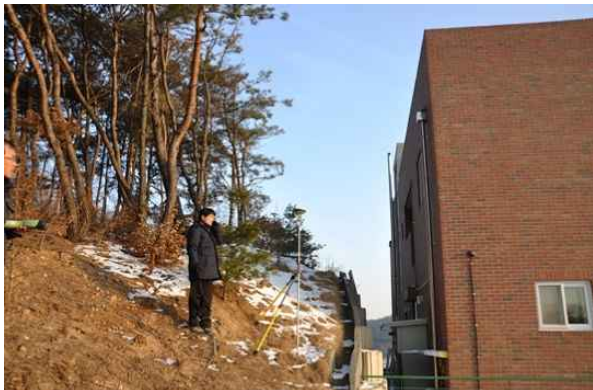
Figure 7. Case of exceeding the allowable error tolerance( \pm 0.07m ) in neighboring areas of land and forest
