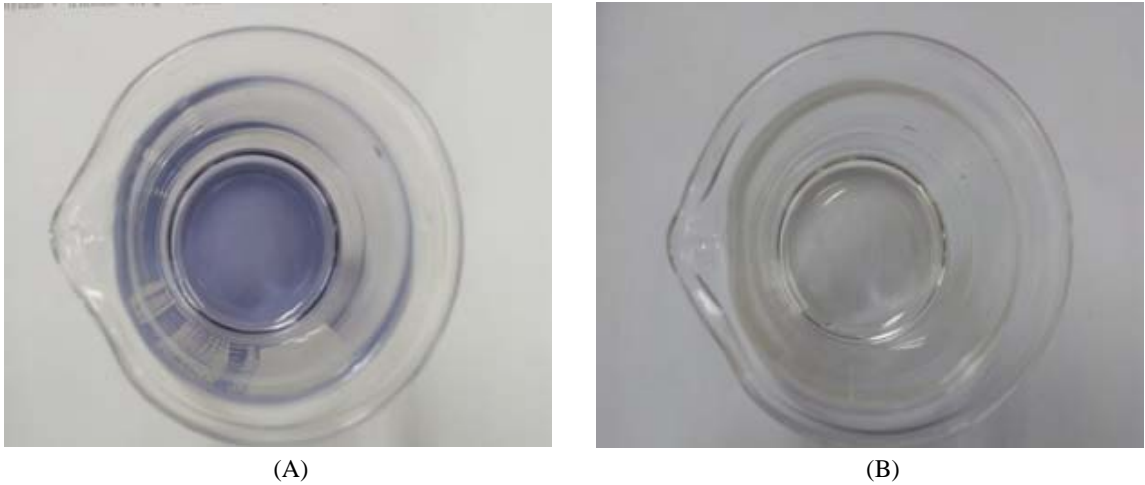
Fig. 12. Changes in color by non-enzyme treatment(A) and enzyme treatment(B) of oxidized starch from water soluble residues.
