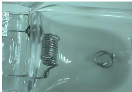
Figure 5. Filament Failure at 18V Test
