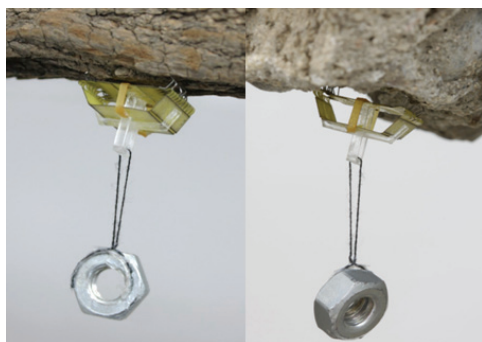
(a) Gripper attached to a tree and stone
