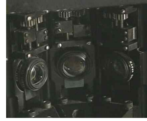
(Figure 3) Cinerama system lens section[4]
