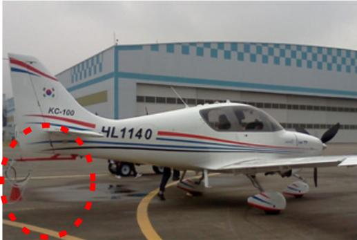
Fig. 5. Trailing Cone Installation
