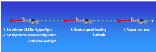
Fig. 6. Level Flight Profile for ADC Test
