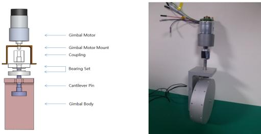
Fig. 5 GMA Design & Manufacture
