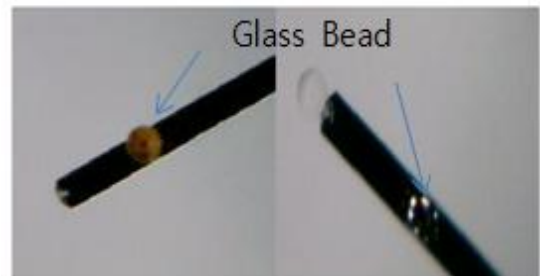
Fig. 12 Attached Glass Bead on Cantilever(Fail)
