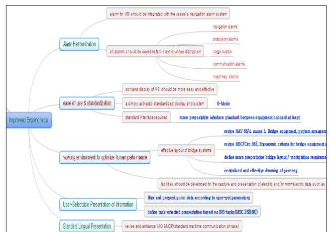
Fig. 3 Example of technical tree for an e-navigation user need, i.e., improved ergonomics
