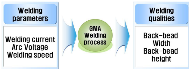
Fig. 4 Welding parameters and geometry on GMA welding process
