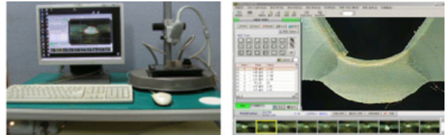
Fig. 5 Measurement of bead geometry
