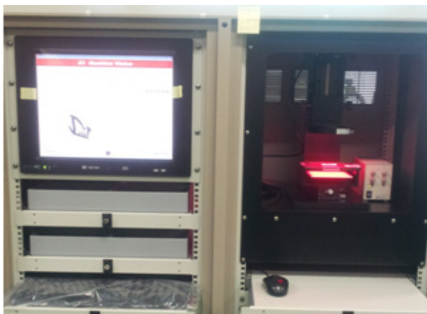
Fig. 4 Developed vehicle sealing inspection system
