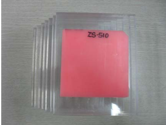
Fig. 3. Mammography phantom: 6 fibers, 5 groups of specks, 5 masses and acrylic plate size: width 12 cm, height 10 cm, thickness 1 cm
