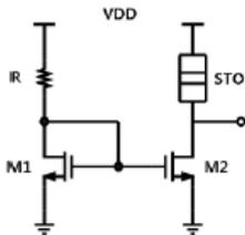
Fig. 4. STO with current mirror circuit.
