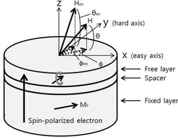
**Fig. 1.** Structure of an STO.
