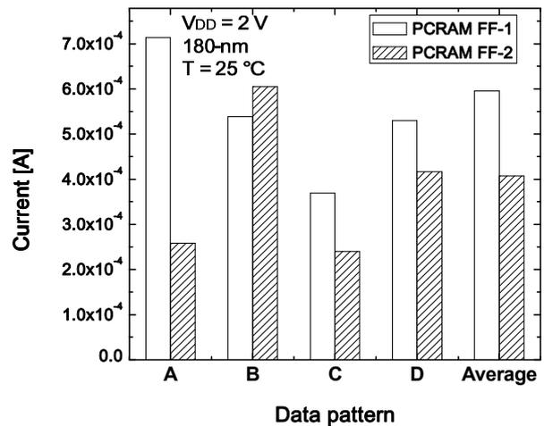
**Fig. 5.** Current consumption of the FF-1 and FF-2 circuits in the storing operation for various data patterns. The data patterns for A, B, C, and D are ‘000000’, ‘101010’, ‘111111’, and ‘11001100’, respectively. Here  $I_{SET}$  and  $I_{RESET}$  are 600  $\mu A$  and 1250  $\mu A$ , respectively. The cycle time for the STORE and RECALL operation is 370 ns.
