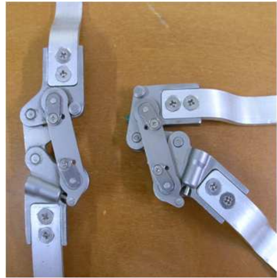
Figure 1. 4-bar linkage orthotic knee joint.
