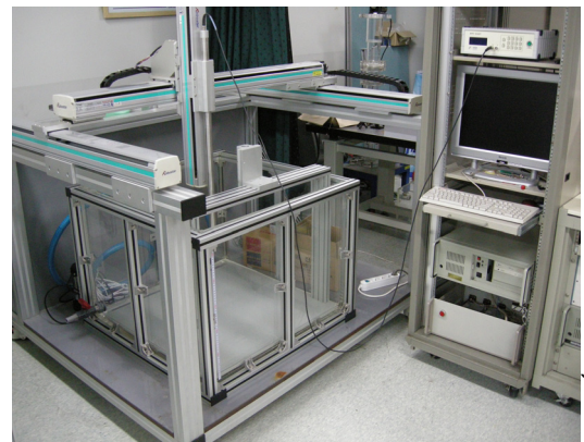
Fig. 5 Photo of ultrasonic scanner system
