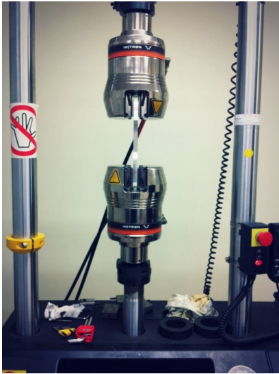
Fig. 3 Photo of Instron 8081 machine for fatigue testing
