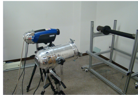
Fig. 3 Infrared thermography system
