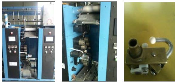
Figure 1. Air-jet texturing machine used in this study.
