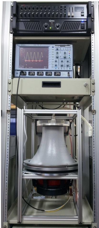
Fig. 7 Photograph of experimental apparatus for flow measurement and generation
